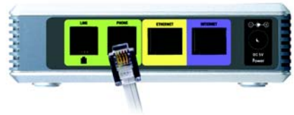
Figure 4-2: Connect a Telephone
